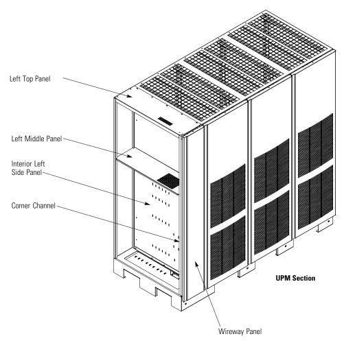
Figure 4-5. Section Joining
